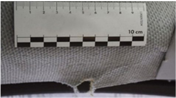
Habillage textile :déchirure, perforation > 5 mm, taches indélébiles
